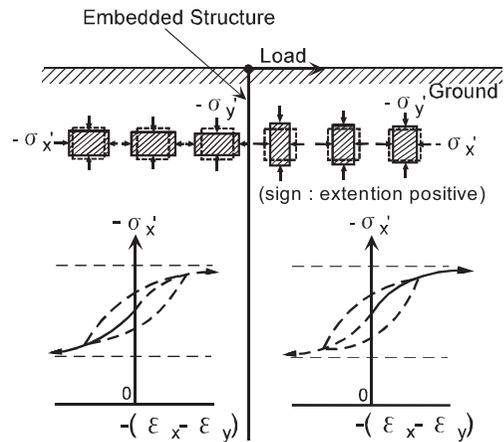
Fig. 2 Hysteretic Subgrade Reaction in Drained Cyclic Shear Condition
