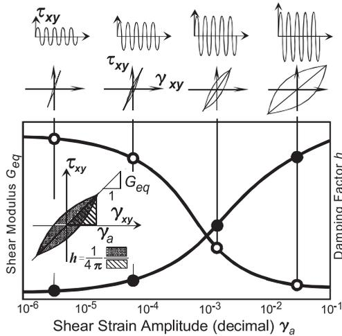
Fig. 1 Sand Behavior under Drained Cyclic Shear
