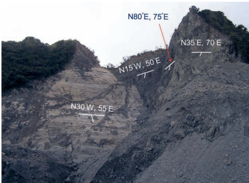
Fig. 4 The landslide scarp. Joint planes were measured remotely. Dip of the joint plane indicated as N15°W, 50°E might be much steeper than 50°. Photo taken on March 24, 2006 by Suwa, H.
