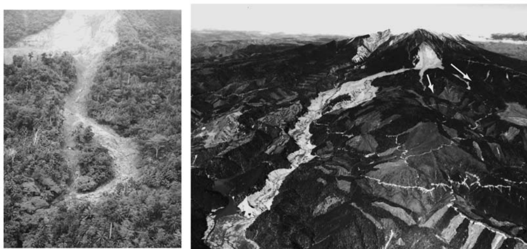
Fig. 10 A portion of debris mass rushing into the neighboring catchment. Left: the 17 February 2006 Leyte slide. Photo taken on March 22, 2006 by Suwa, H. Right: the 14 September 1984 Ontake slide. Modified from the photo taken on a day of October, 1984 by Pasco Co. Ltd.
