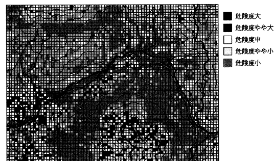
Fig. 15 The slope failure risk predicted by Type 2
