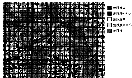
Fig. 16 The slope failure risk predicted by Type 3
