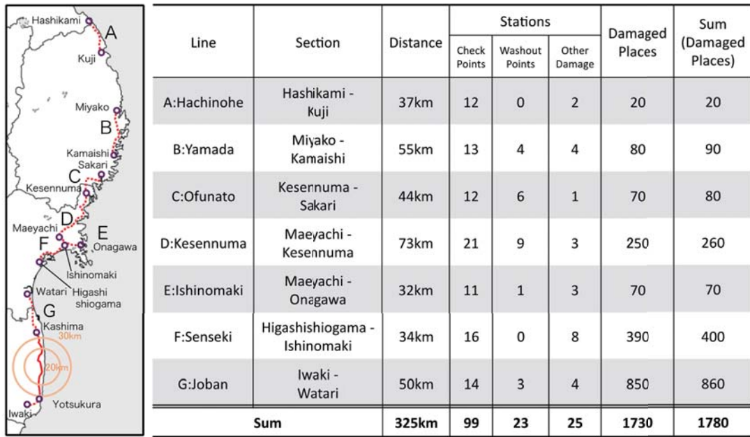
Fig. 3. Damage to railway caused by the tsunami (JR East)
