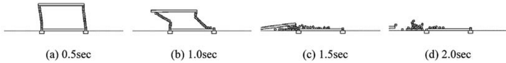
Fig. 9 Behavior of 1-story structure for the joint strength of 0 \text{ N/m}^2 (lateral pressure: 5.0 KPa)
