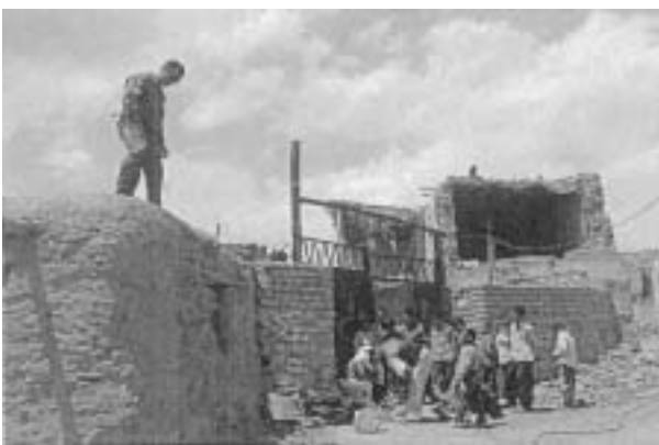
Photo 10 Forced vibration test on the adobe house
