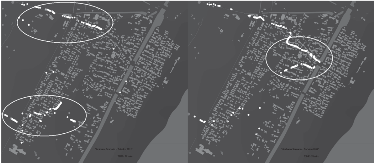
Figure 13 Representative snapshots of two different repetitions of simulation. Bottlenecks can be observed in the circled areas. Near the exit points, the evacuation building and a bridge connecting two areas are separated by a channel.
