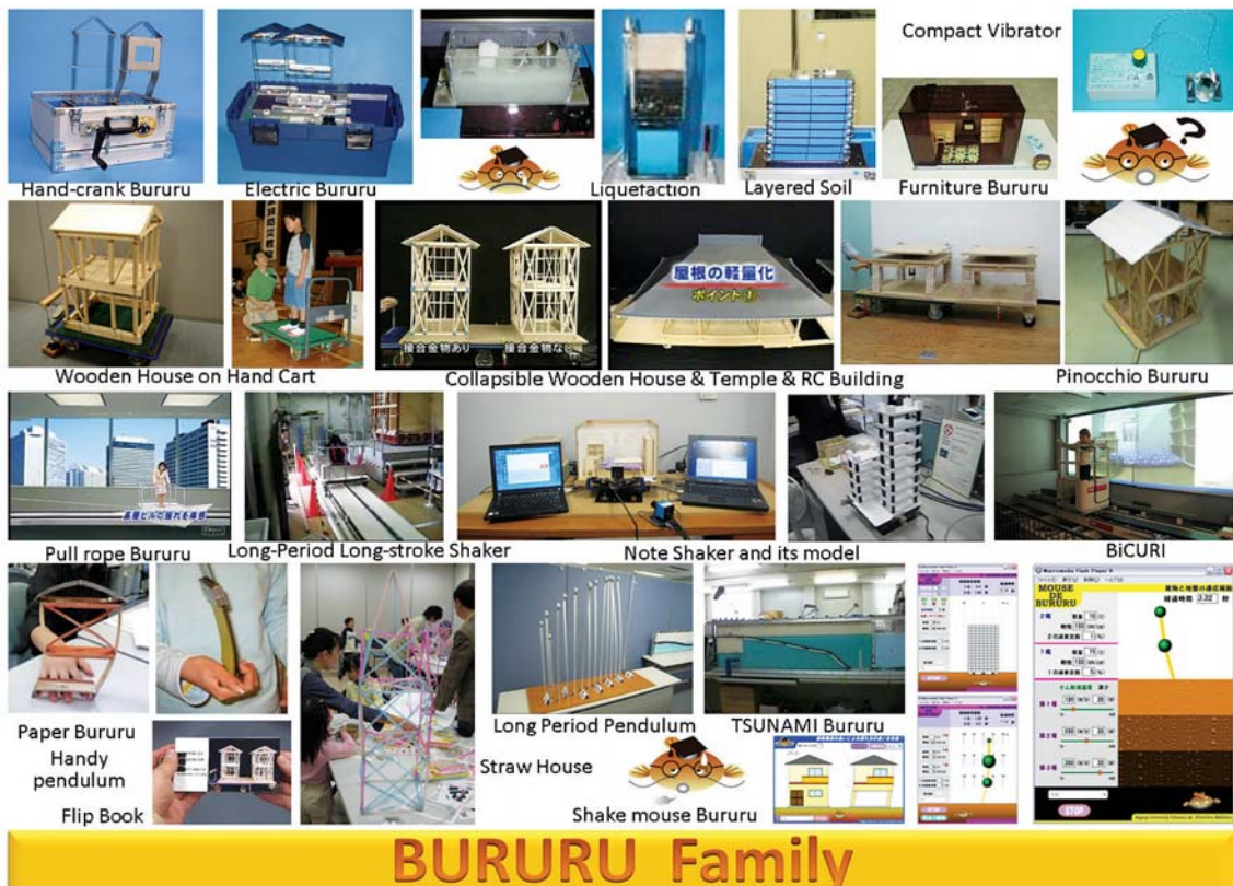
Figure 6: The “BURURU” family, which consists of a series of educational devices that demonstrate earthquake-related vibrations and other phenomena in ways that assist disaster mitigation training activities.
