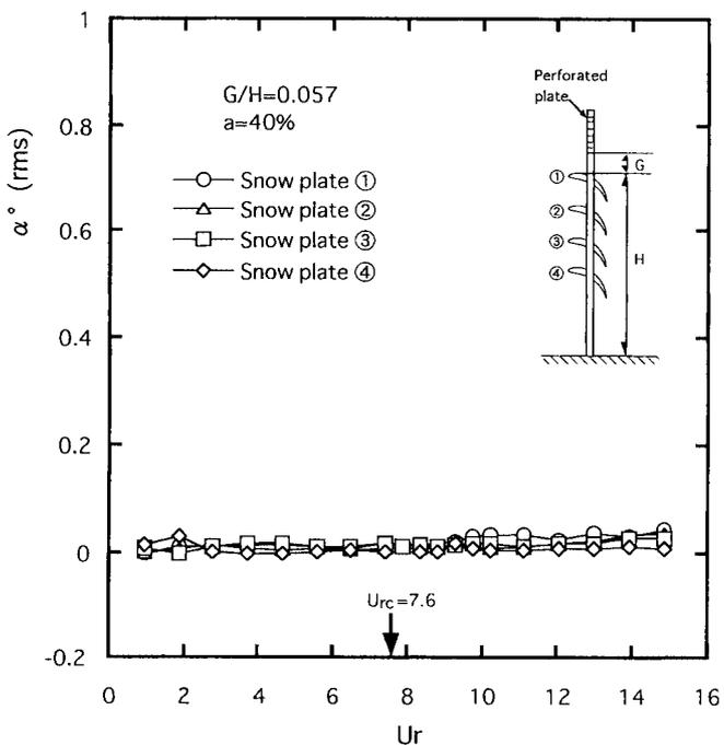
Fig. 17 Response of each snow plate when a perforated plate is attached to the topmost part of the snow fence
