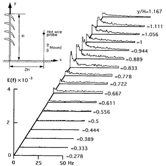
Fig. 13 Power spectrums of fluctuating velocity behind the snow fence (with perforated plate)
