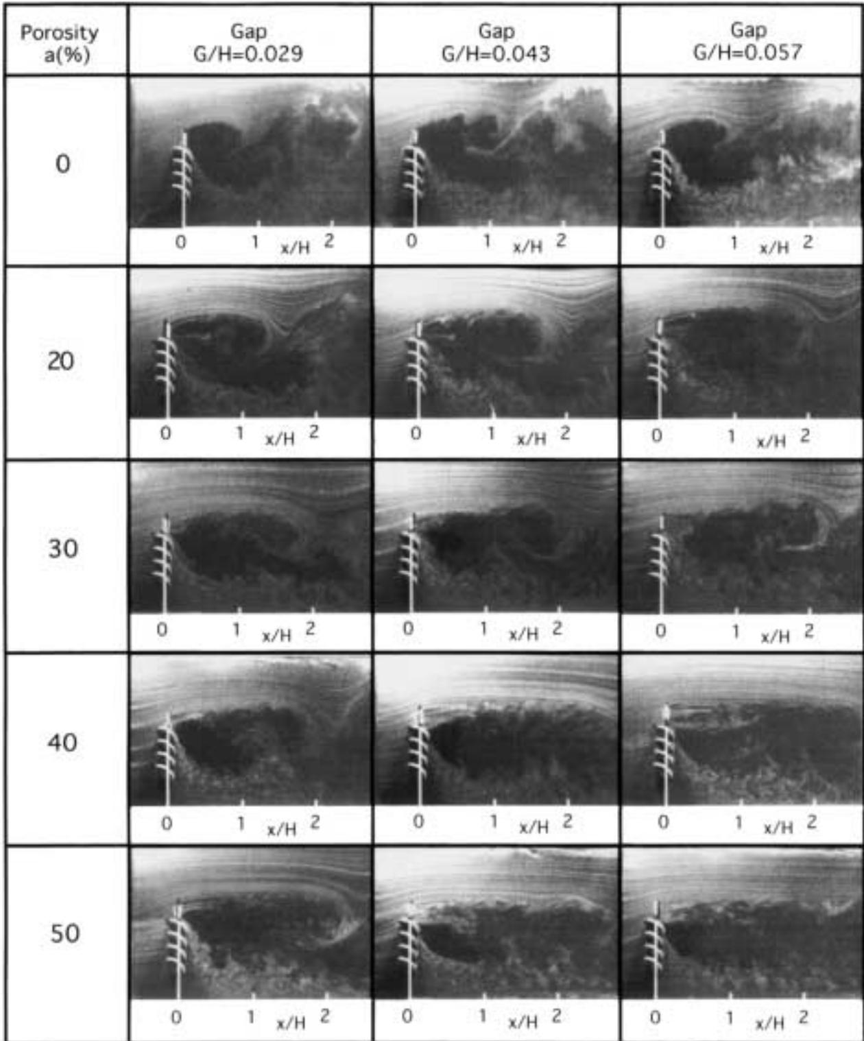
Fig. 10 Visualization of the flow pattern around the snow fence with a perforated plate attached to its topmost part
