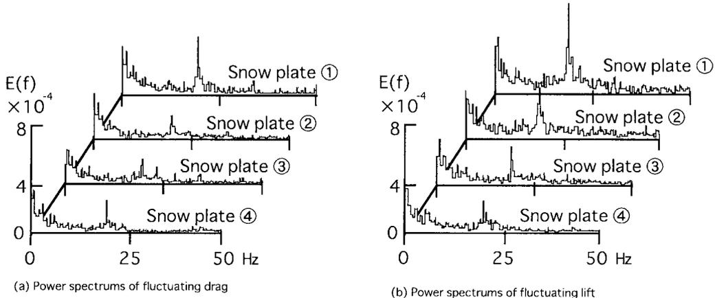
Fig. 8 Power spectrums of fluctuating drag and lift of the airfoil snow plates
