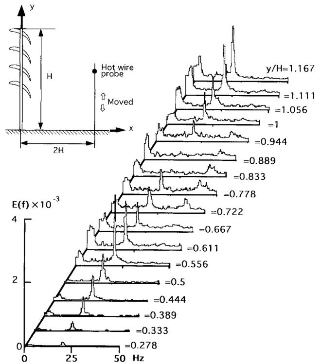
Fig. 9 Power spectrums of fluctuating velocity behind the snow fence
