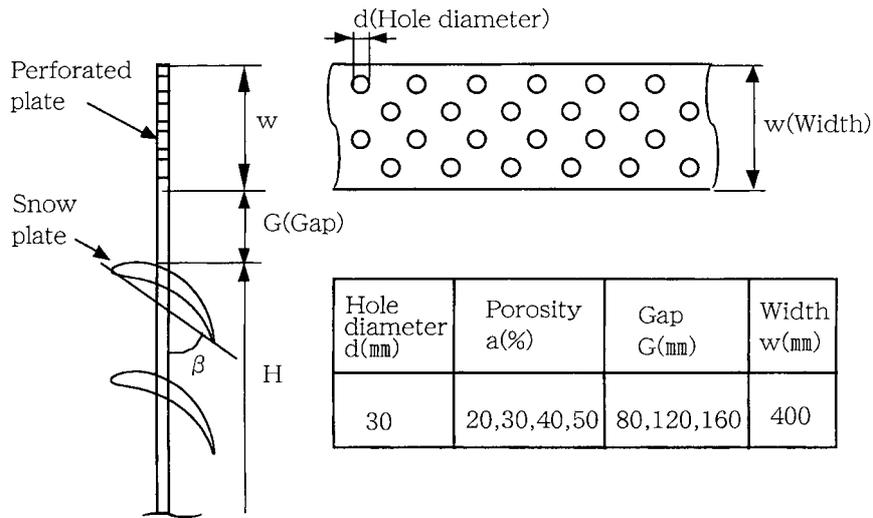
Fig. 3 Perforated plate for snow flow control
