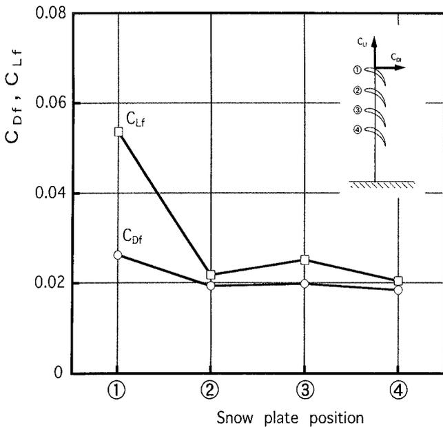
Fig. 7  $C_{Df}$  and  $C_{Lf}$  of each snow plate
