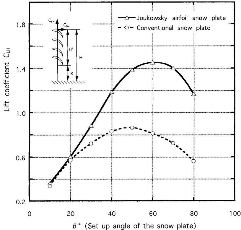
Fig. 5 Lift coefficient,  $C_{LH}$ , of the snow fence versus the set up angle,  $\beta$
