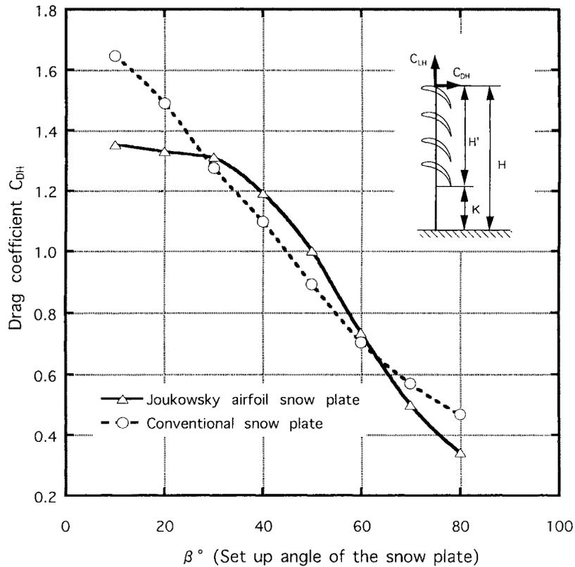
Fig. 4 Drag coefficient,  $C_{DH}$ , of the snow fence versus the set up angle,  $\beta$
