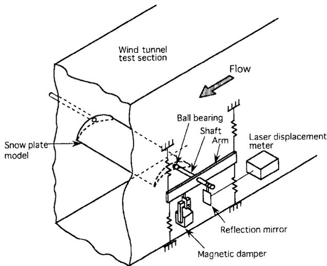
Fig. 2 Schematic diagram of the free-vibration apparatus
