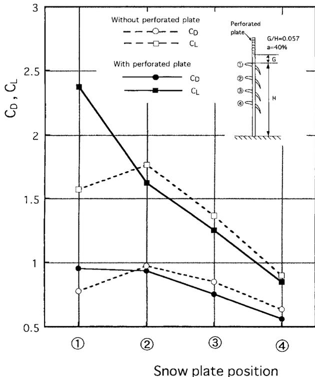
Fig. 14  $C_D$  and  $C_L$  of each snow plate when a perforated plate is attached to topmost part of the snow plate
