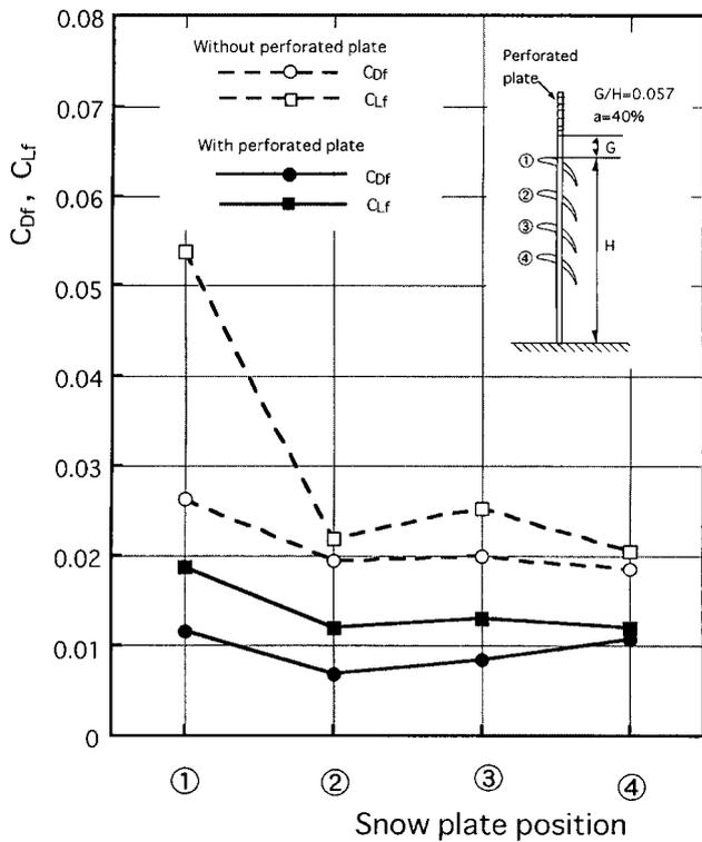
Fig. 11  $C_{Df}$  and  $C_{Lf}$  of each snow plate when a perforated plate is attached to topmost part of the snow plate
