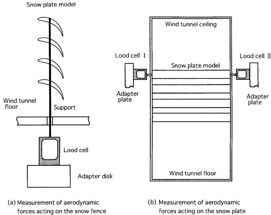
Fig. 1 Load cell apparatus for measuring of aerodynamic force acting on the snow fence and snow plates
