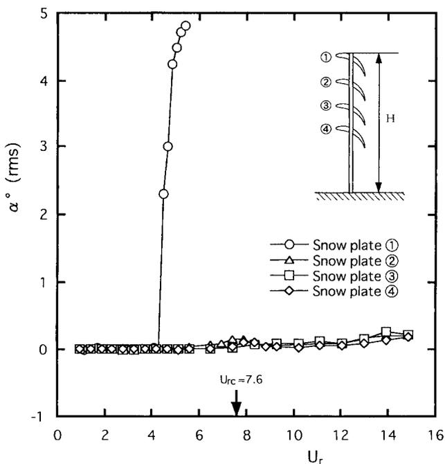
Fig. 15 Rotary oscillation response of each snow plate in the absence of a perforated plate
