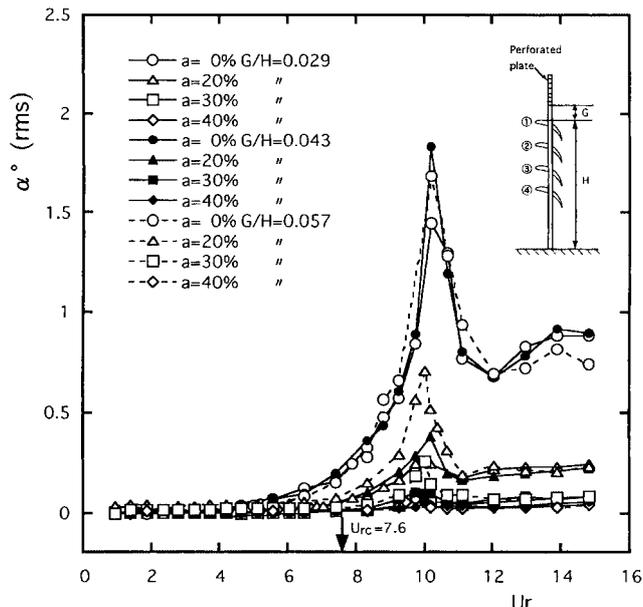
Fig. 16 Rotary oscillation response of snow plate number ① when a perforated plate is attached to the topmost part of the snow fence
