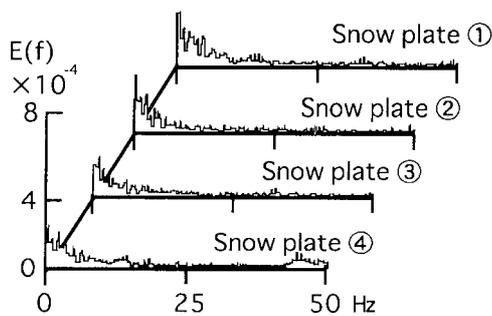
(a) Power spectrums of fluctuating drag
