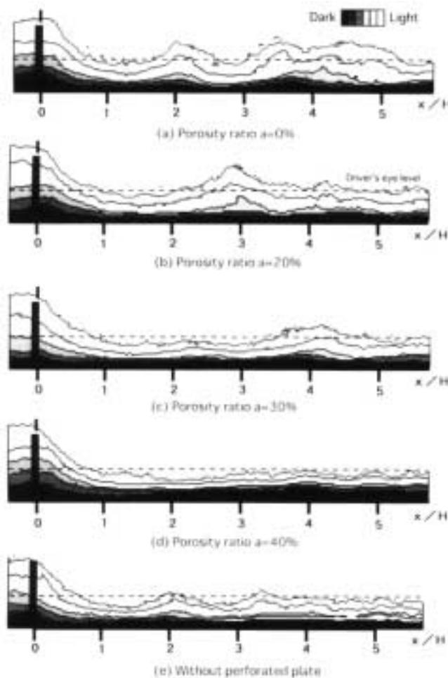
Fig. 18 Density distribution of blowing snow for the snow fence with a perforated plate
